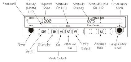
Dual concentric knobs on the right side are used to select squawk codes and change altitude values. Turning the large, outer knob moves the cursor to allow editing of the selected character. Turning the small, inner knob changes values.
