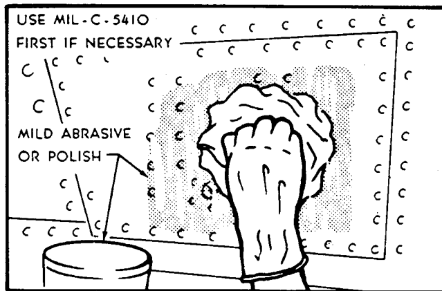
FIGURE 6-12. POLISHING AND BRIGHTENING ALCAD SURFACES
